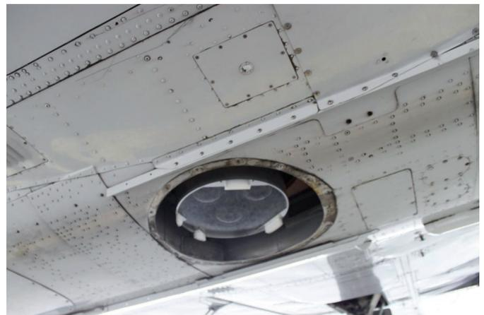
B66 Aerial Surveillance camera installed in an aircraft
