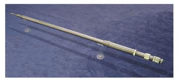
the tip of the endoscope to be cooled to < 200°C and the positive pressure to provide enough airflow to keep the prism clean. In addition, to stop the endoscope transmitting heat from its tip to the connected camera – special heat breaks were designed into the body so that the camera end of the endoscope was kept below 50°C.
