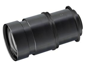
Model 357 provides high image resolution and minimum geometric distortion from 400 to 770 nm, and can image objects from 800 mm to infinity without using add-on adapters. When focused at infinity, the lens achieves high image resolution on axis at full aperture throughout the zoom range without refocusing.
