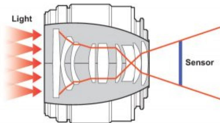
There are various factors that govern the size of an optical system and for the purpose of this article we consider the design of a fixed focus lens. The key factors that affect the size of a fixed focus lens are the sensor it is designed for plus the aperture or f number, focal length and resolution required to meet the requirements of the target application(s).
