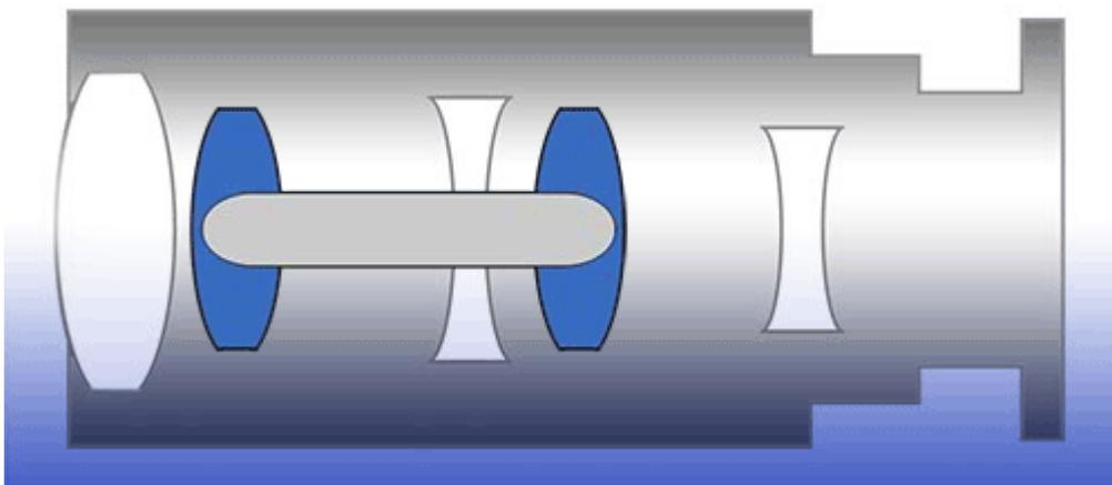
In this new design there are two groups of elements that move together in relation to a middle group. The movement is linear so there is no requirement for complex cam profiles. The optically corrected zoom lens beneficially also maintains focus and resolution throughout its zoom range. We are looking for partners to 'road-test' our new optically compensated zoom lens. If you would like to know more please send us details of your target application in this [attached form](#).
